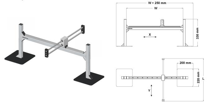
Custom cut linear guiding system mounted on high density aluminum profile for X-travel and a rigid custom sized double-arm boom creates requested Y-travel range of the Digital Microscope. The height of the linear guide can be adjusted and set to give the correct working distance of the Digital Microscope using 4x angle brackets.
