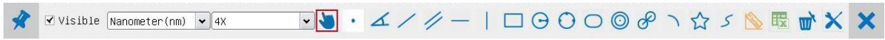
Figure 8 - The Measurement Toolbar Button on the Upper Side of the Video window
