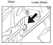
Insert the Slider's pin to the oval shape hole
